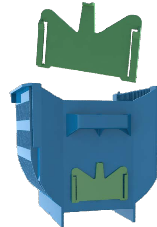
CARD HOLDER-R.1 Welded to Process Boat
